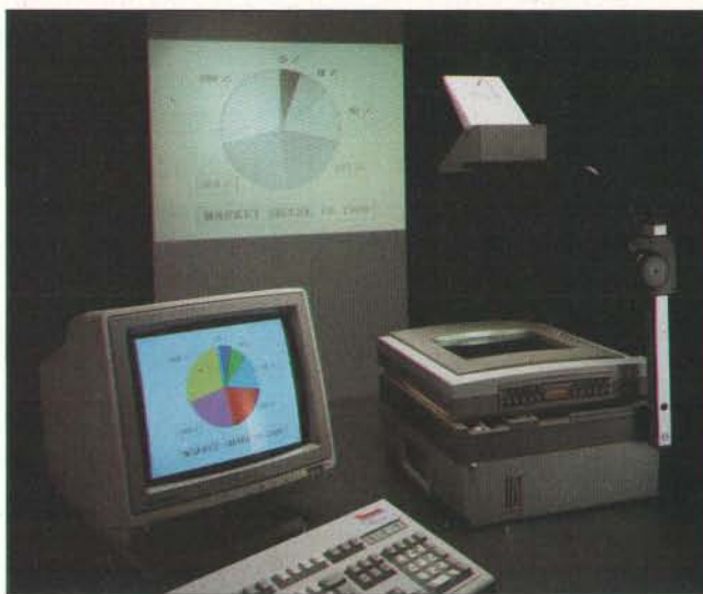
With Datashow 480, you can project PC-generated images on a large screen with an overhead projector.
